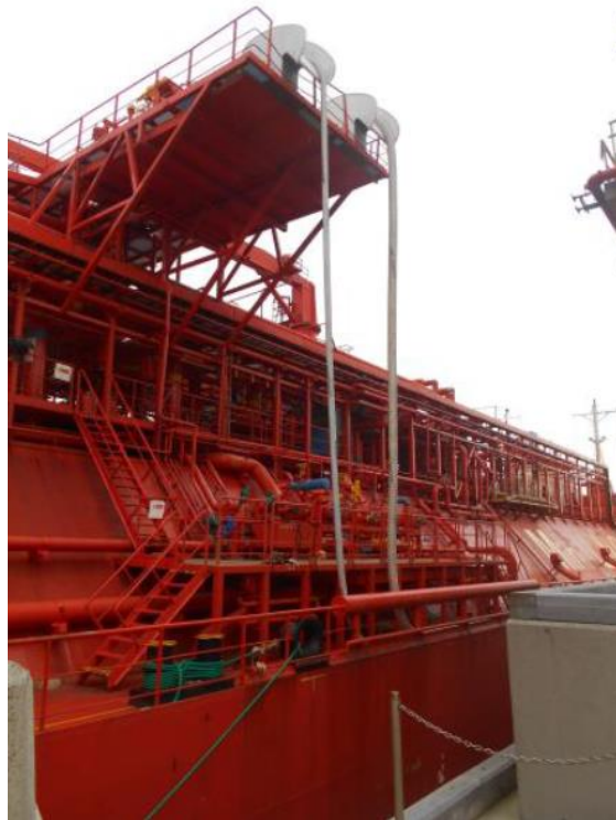
Picture 5. Hose arrangement on the MV Coral Fraseri.
