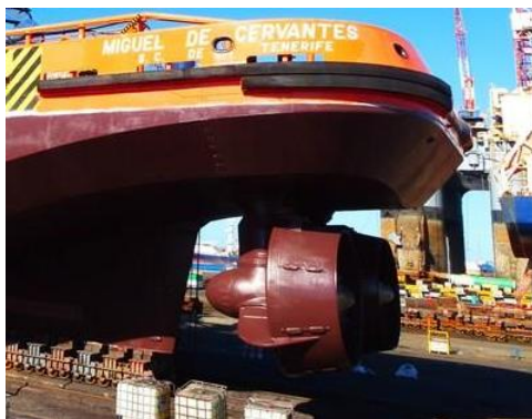
Figure 56. Azimuth propellers installed on the stern. Source: SASEMAR (left) and SCHOTTEL (right).
