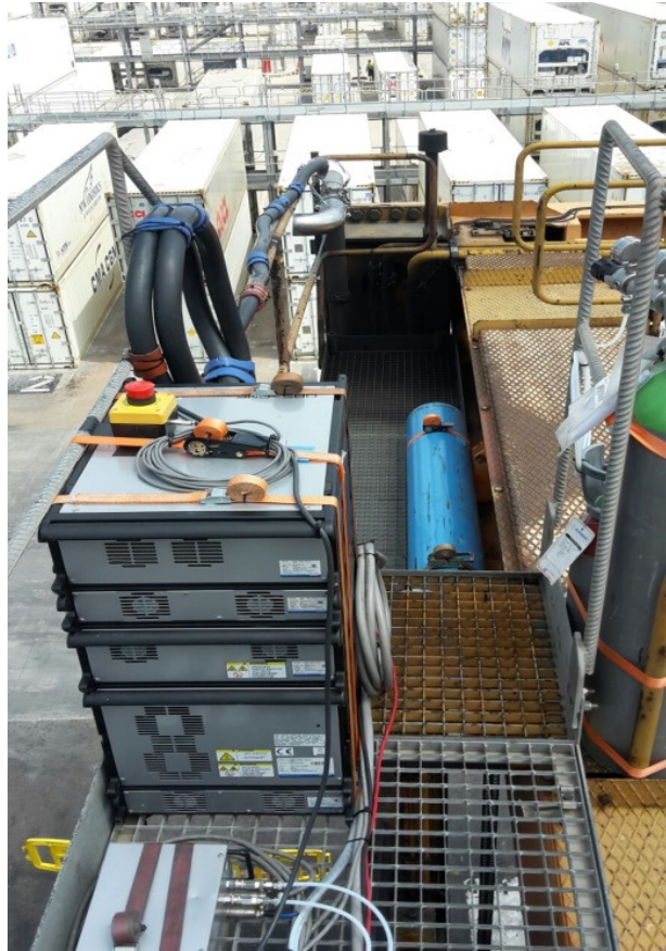
Figure 8. Air gas bottle installed laying down on the floor
