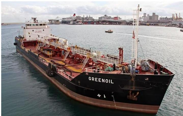
Designed for 4 x 300m<sup>3</sup> LNG tanks
