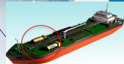
Virtual image of the barge with the two tanks added in the deck (the image shows 50m³ tanks)
